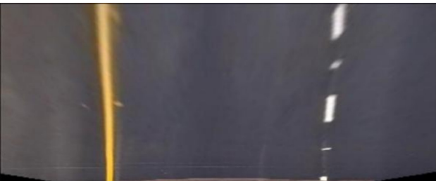
(a) (b) 透视变换后直线检测
